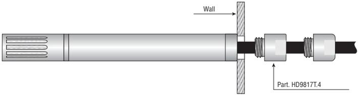
The wall can be 2mm thick at most while the hole in the wall can be 10.5mm.
